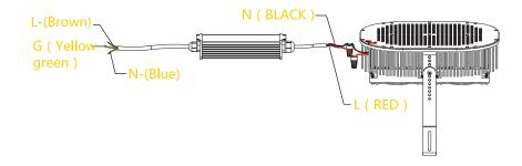
Properly cap-off the second set of Line and Neutral input wires on the 280W/350W MUR head.
