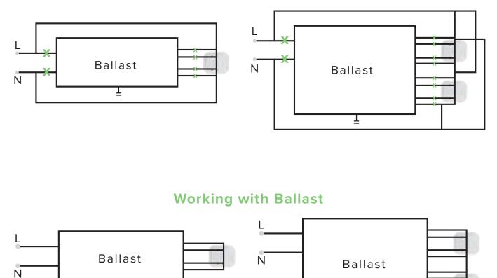
**STEP 4:** If lamp fails to operate (no light output, flickering, or low light output) after restoring power back to the fixture it is recommended to follow below wiring diagram to bypass the ballast and run direct voltage to sockets.
