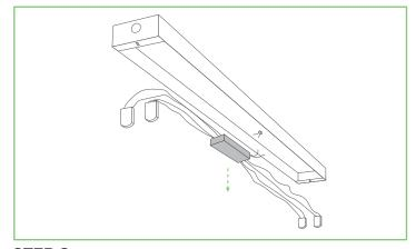
**STEP 3:** Disconnect old ballast from AC and remove the ballast and tombstones.
