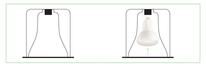
**STEP 3:** Install the ESL Vision PL lamp into existing socket.
