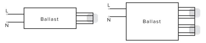
STEP 4: If lamp fails to operate (no light output, flickering, or low light output) after restoring power back to the fixture it is recommended to follow below wiring diagram to bypass the ballast and run direct voltage to sockets.
