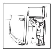
**STEP 4:** Replace the reflector and lens carefully by reversing procedure used to remove it.
