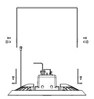
Install the L-brackets to the fixture.
