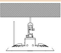
3 Attached the fixture hook to a pre-installed ring in the ceiling. Install the provided screw into the hook.
