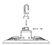
First install the hook to the RHB fixture using the provided screws to mount to the hook to the fixture.
