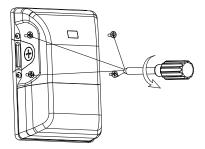
4. Screw the bottom mounting plate to the wall
