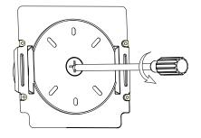
5. Fix the bottom plate on the round plate
