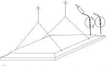
2 Ensure that the power is turned off at the breaker. Connect power to the driver as show in Wiring Diagram 1.
