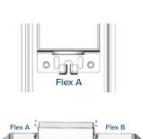
Insert the high-voltage side (Flex A) of the emergency power into the bracket slot. Then fix the emergency battery to the supporting bridge by using two screws on Flex B side and two screws on Flex A Side.  $2^{\rm Install}$  the EM supporting bridge on the back plate and screw in A1/A2/B1/B2 and wiring.
