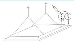
Ensure that the power is turned off at the breaker. Connect power to the driver as show in Wiring Diagram 1.
