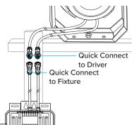
5 Connect to the fixture using the Quick Connect cables.
