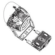
2 Slide the driver box onto the bracket.
