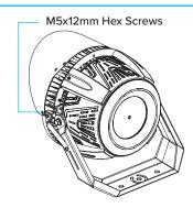
4 Fasten the light barrier to the fixture body using the M5x12mm hex screws.
