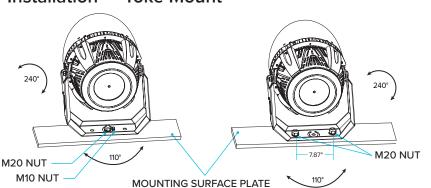
Place SPT Series fixture on mounting surface plate. Tighten the fixture to the mounting plate using the M20 and M10 screws (do not tighten down fully). Adjust the fixture to it's desired position vertically (240°) and horizontally (110°).
