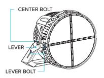
To adjust the angle loosen the center bolt and the two lever bolts, adjust the angle of the fixture, and then tighten the center bolt and two lever bolts.
