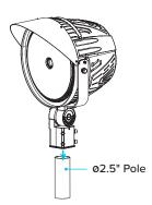
Mount the SPT Fixture to the Slip Fitter Mount. Place the fixture onto the mounting pole.
