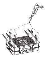
Attach stints to the external driver Attach stinus to the con-box with the M6 16mm screws
