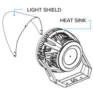
$\mathbf{3}^{ ext{Place}}$  the light barrier on the fixture body.
