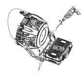
3 Secure the driver box using the M8 20mm screws
