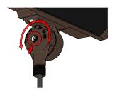
$3^{\text{To aim}}$  the fixture, use a hex key to loosen the screw. Move the fixture head to the appropriate position and tighten the screw to lock it in position.
