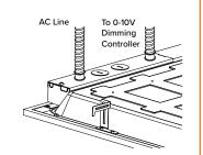
**4** Connect the AC line (L, N and GND) to the LED Driver using 18–14AWG wire as shown in **Wiring Diagram 2**.
