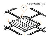
Insert into ceiling grid. Secure safety cable to connection hole as needed according to local building codes.
