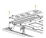
Remove enclosure cover and remove knockout for AC input and 0–10V control lines. Install fittings in knockout holes if needed.
