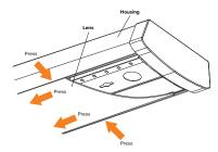
Install the lens starting at one end of housing. Insert the lens into the slot on one side of the housing. Carefully bow the lens into curve to slide the opposite edge into the slot. Continue this action down length of the lens until it is fully installed onto housing.
