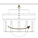
Plug in the sensor and twist clockwise to lock in place.
