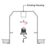
2 Thread the socket adapter into the socket.
