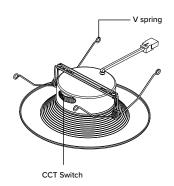
Set the CCT switch to your desired color temperature. If installing into a 5" housing adjust the V spring to suit. If installing into a 6" housing no adjustment is needed.
