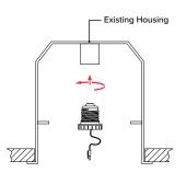
Thread the socket adapter into the socket.
