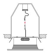
3 Plug the female connector of the retrofit into the male connector of the socket adapter assembly.
