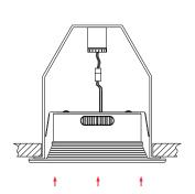
A Squeeze both spring arms together and insert into the slots of the can. Tuck all wires into the can and carefully push the retrofit downlight into the can housing.
