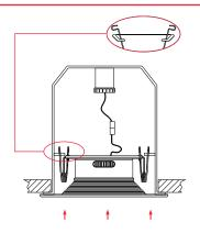
A Squeeze the spring arms together and insert into the slots of the can. Tuck all wires into the can and carefully push the retrofit downlight into the can housing.
