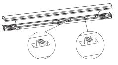
Adjust kelvin and wattage as desired using the dip switches located on the driver. Close LED assembly.
