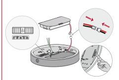
a) Open the battery hatch using the thumb locks and take out the battery pack. Plug in the battery pack. Replace the battery pack and push to close. b) Select desired kelvin.
