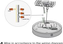
$4^{\rm Wire in accordance to the wiring diagram.}_{\rm (See below)}$
