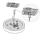
Attach steel safety wire onto bracket.
