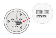
Using the switch on the back, select the desired kelvin.
