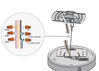
$\begin{tabular}{ll} 4 \text{ Wire in accordance to the wiring diagram.} \\ 4 \text{ (See below)} \end{tabular}$
