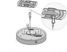
$3^{Attach}$  steel safety wire onto bracket.
