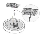
Attach steel safety wire onto bracket.
