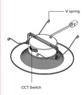
Set the CCT switch to your desired color temperature. If installing into a 5" housing adjust the V spring to suit. If installing into a 6" housing no adjustment is needed.
