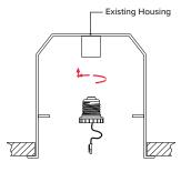
Thread the socket adapter into the socket.
