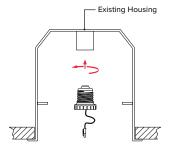
2<sup>Thread</sup> the socket adapter into 2<sup>the</sup> socket.
