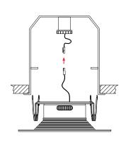
**3** Plug the female connector of the retrofit into the male connector of the socket adapter assembly.
