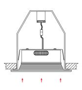
A Squeeze both spring arms together and insert into the slots of the can. Tuck all wires into the can and carefully push the retrofit downlight into the can housing.
