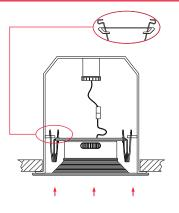
4 Squeeze both spring arms together and insert into the slots of the can. Tuck all wires into the can and carefully push the retrofit downlight into the can housing.
