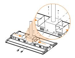
3Put wires back into junction box, install side panels with supplied screws (x2).
