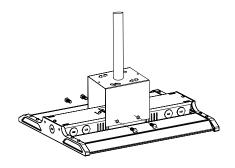
$2^{\text{Mount fixture to junction box bracket with the}} \\ \text{supplied bolts (x4), connect wires to fixture.}$
