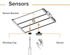
Use a screwdriver to remove the shorting cap, then screw in the optional sensor kit.
