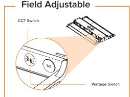
The fixture has 3 selectable CCTs and 3 selectable wattages. Adjust as needed.
