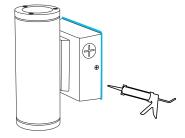
4 Seal the fixture where it contacts the mounting surface with a silicone sealant. Turn the supply power on and test the fixture to ensure that it functions properly.
