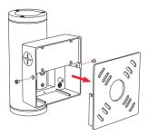
Remove the two set screws and save for later use, then separate the junction box bracket.
