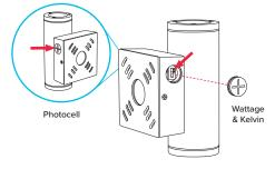
Remove the side access plugs to access the Wattage and Kelvin dip switches, and the integrated photocell. Slide each switch to the desired setting and replace the plug securely.
