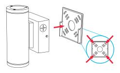
Mount the junction box bracket. Wire the fixture according to the Wiring Diagram below. Place the fixture on the bracket, replace the set screws and secure.
