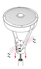
Position fixture on post top tenon or pipe. Tighten down all 8 allen head set screws to 6 ft-lbs (72 in-lbs).
