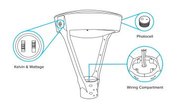
Kelvin & wattage adjustment, the photocell receptacle, and the wiring compartment are easily accessed via side access plugs on the body of the fixture.
