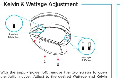
With the supply power off, remove the two screws to open the bottom cover. Adjust to the desired Wattage and Kelvin and select your Up Only / Down Only / Up & Down lighting distribution by sliding the switches on the controllers inside. Replace the cover and fix it in place with the screws.
